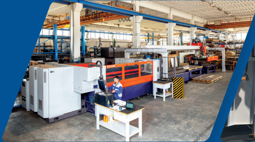
Laser Bystar 3015 4000w maximum resonator power, cutting thickness 20 mm
