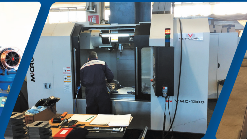
"MICROCUT" VMC - 1300/40 Table dimensions 1500 x 660 mm with permissible load up to 1200 kg
